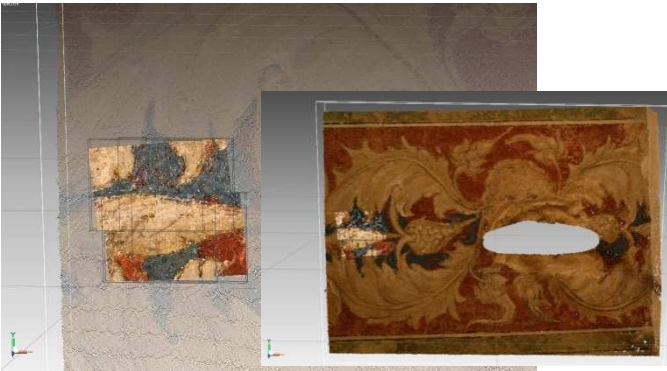
Figure 1. 3D RGB point clouds general 951000 points and detail of 2 million points
